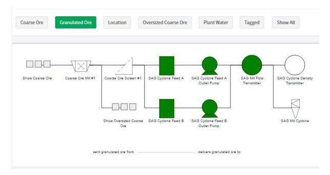
In the diagram above, we are looking at the path that granulated ore takes from our ore mill, through the processing system.
