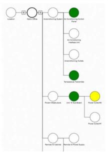
To the left is an example diagram from ARDI. It begins at the office, then splits into various sub-systems, such as airconditioning, power etc.
